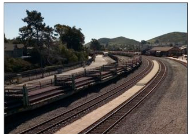
A train of special-purpose cars carrying welded rail at San Luis Obispo in February 2022. One imagines the workers and observers of 1926 being impressed with the lengths, weight (probably 136 rather than 90 pounds per yard), and mechanized handling of today’s rails.
