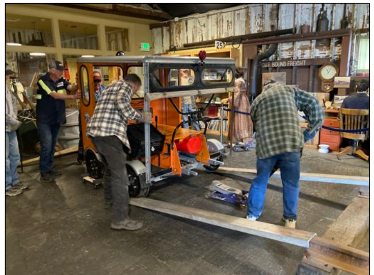
Above, wheels on wheels. Dollies helped maneuver without damaging the floor. Aluminum channel ramps provided transition to the display track, below.
