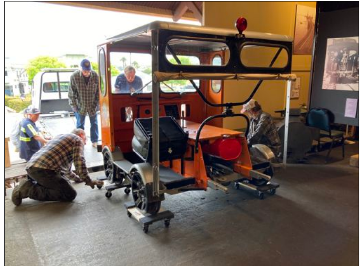
Above, wheels on wheels. Dollies helped maneuver without damaging the floor. Aluminum channel ramps provided transition to the display track, below.
